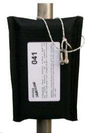
**ATTENTION :** If the antenna side is not installed towards sky position or covered by other objects transmission may not work properly.
