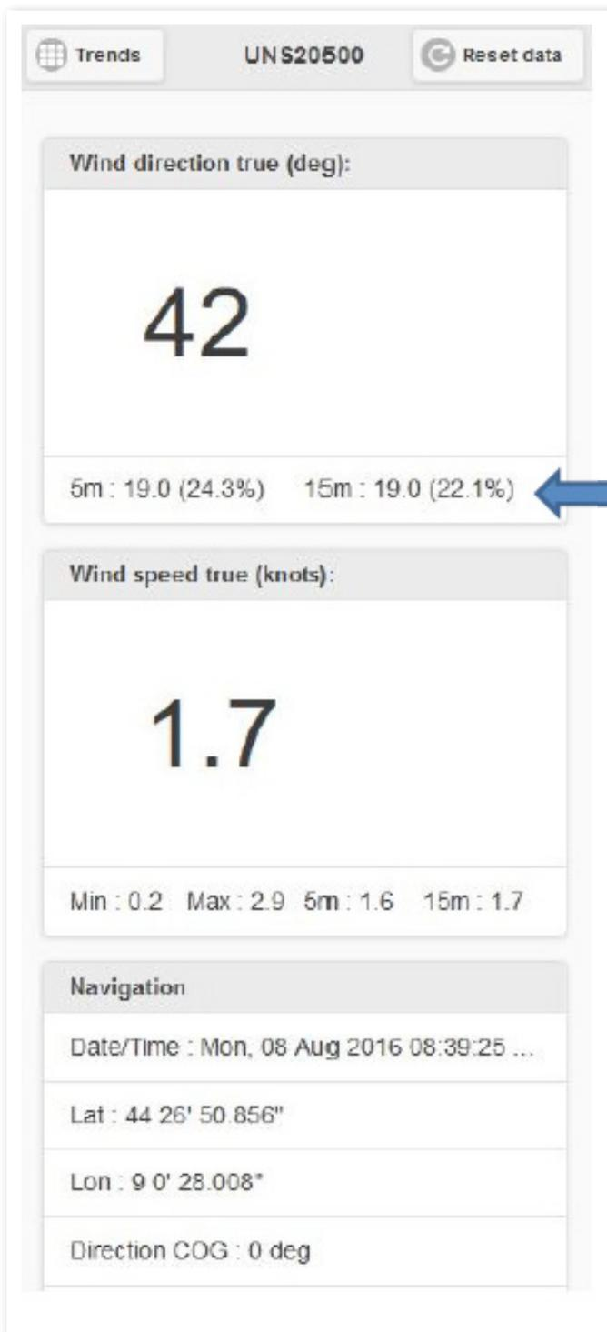
The main wind monitoring page shows the current true wind direction and speed combined with several statistics.
